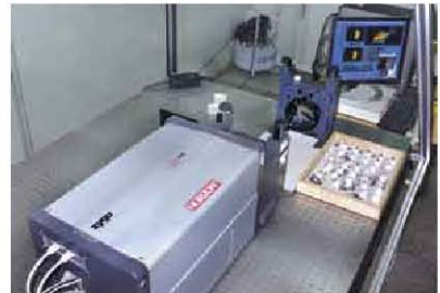
The ZYGO Interferometer Batch testing of Horizon Prisms
